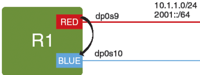
Figure 7. Route leaking between routing instances
